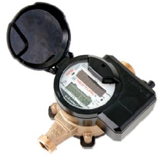
Open the cover to expose the face of the meter. The LCD display is light activated. Shine a flash light over the light sensor for several seconds and the LCD display should appear, showing your current read.
